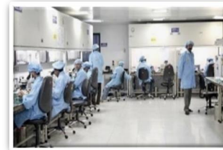
Clean Rooms - Class 10K
